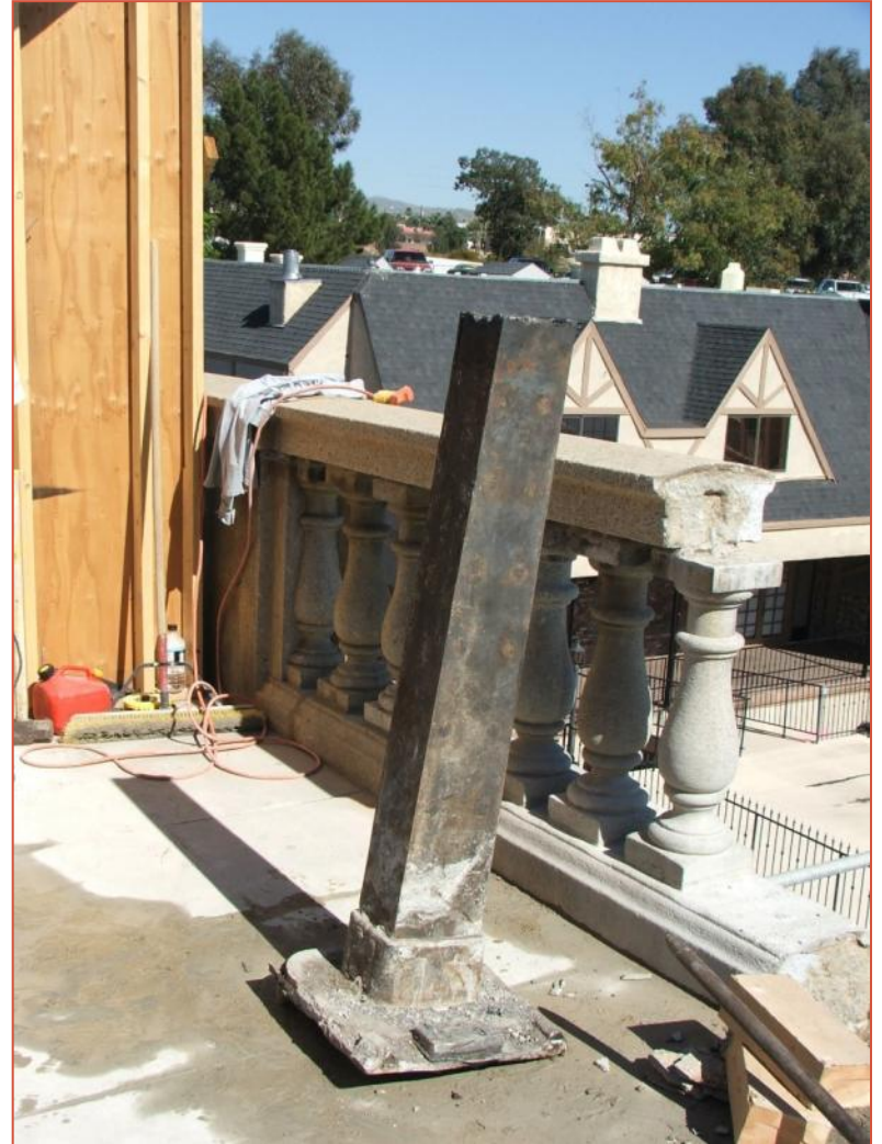
Cause of problem – removed rusted lamp support post
